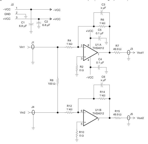
Figure 1–5. THS4012 EVM Schematic — Differential Input (Inverting Operation)
